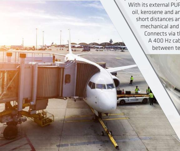
Boarding bridges are closed walkways connecting airport gates to the airplane to facilitate passenger boarding and disembarking. One end anchors to the airport building with the opposite end free to anchor to different models of aircraft. Bridges speed up operations, reduce aircraft downtime, simplify passenger flow, and facilitate access for children and the disabled.
