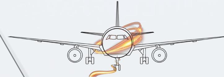
Our flagship 400Hz cable powers aircraft from the ground when at rest, parked on the runway or in hangars.
