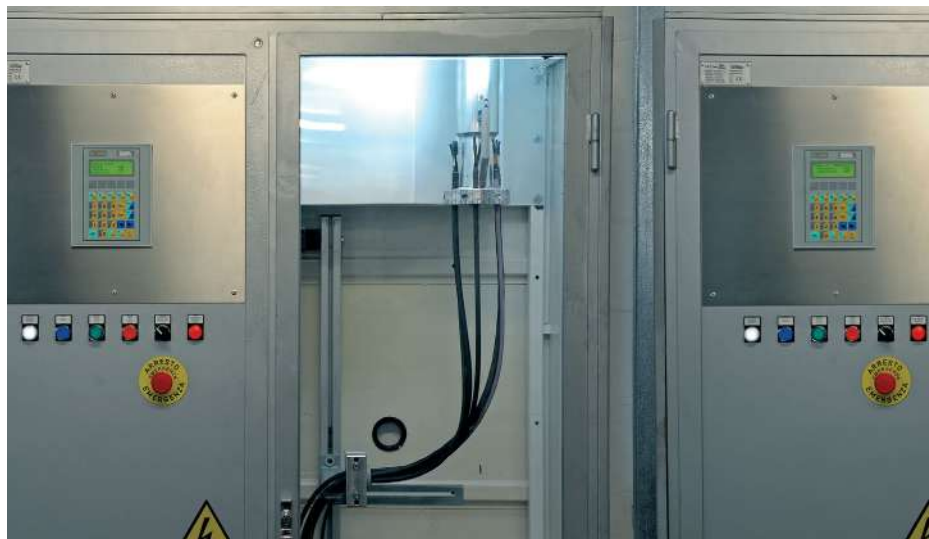
TORSION SIMULATOR – ANGULAR SPEED 20 RAD/s 2 ANGULAR ACCELERATION 30 RAD/s 2
