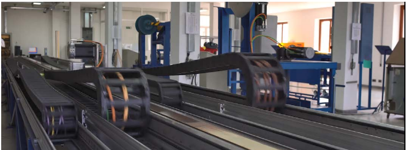
CHAIN WITH A LENGTH OF 18 m – TOP SPEED 200 m/min – MAXIMUM ACCELERATION 10 m/s 2
